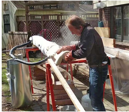
Greg Decker steamed freshly cut white oak planks to 212 degrees and approximately 25- 30% moisture content to form curved bases for four benches
