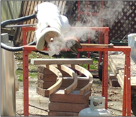
Greg Decker steamed freshly cut white oak planks to 212 degrees and approximately 25- 30% moisture content to form curved bases for four benches
