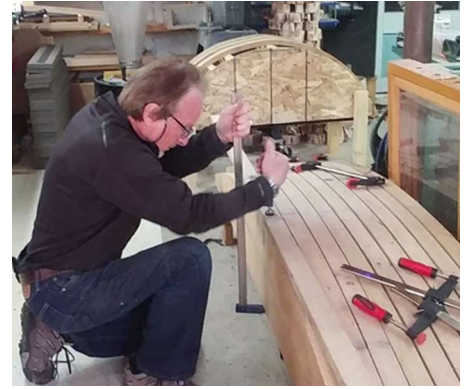
Greg Decker steamed freshly cut white oak planks to 212 degrees and approximately 25- 30% moisture content to form curved bases for four benches
